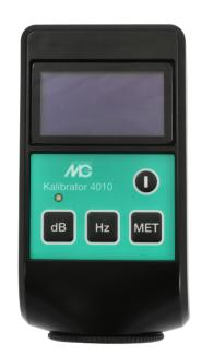
The 4010 is a sound calibrator conforming to IEC 60942 class 1 and ANSI S1.40 for the calibration and the verification of microphones and sound level meters. The combination of two sound pressure levels and two frequencies allow both level linearity and frequency linearity to be verified. Each sound calibrator is supplied with an individual calibration certificate.
